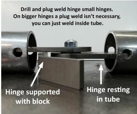
4. Assemble hinge pieces with brass washer. Slide hinge in a tube, use extra piece to hold top hinge side, then slide into second tube. Pictured to the left. Plug weld hinges to tubes.
